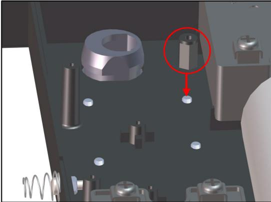
Place the board on the supports and secure it with the other four M3 screws provided.
